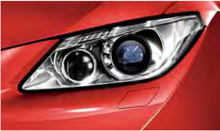
Bi-xenon headlights with AFS (Adaptive Front-lighting System).
