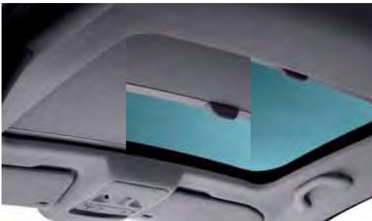
Interior and exterior view of the panoramic glass sunroof (in lieu of roof rails on Ibiza ST).
